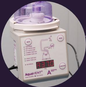
**2** | Autofill Humidification Chamber maintains water level when using a bag of sterile water.
